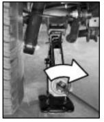
Rear Flat Tire: Place the jack under the curved rear axle pad. Make sure the jack head is positioned so that the rear axle pad is resting securely on the jack head.
